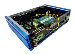
Connect the MS-99C0's cable to the LVDS connector on the motherboard. Make sure the cable is inserted in the right direction.
