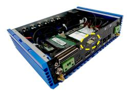
2. Secure the MS-99C0 LVDS to DVI-I Converter Board to the system rear panel with two hexagonal screws.
