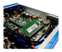
Push the memory gently downwards until the slot clips click and lock the memory in place.
