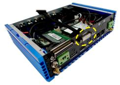
Connect the LVDS cable to the LVDS connector on the motherboard. Make sure the LVDS cable is inserted in the right direction.
