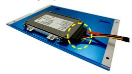
5. Connect the SATA signal & power cable to the motherboard.
