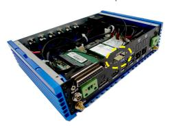
Secure the LVDS cable to the system rear panel with two hexagonal screws.
