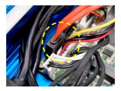
6. Align the notches and replace the system cover.
