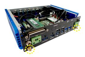
4. Fasten the rear panel back to the system with screws.
