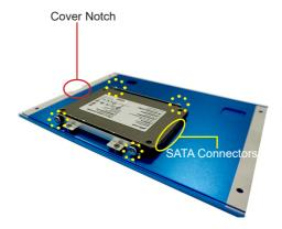
4. Connect the SATA signal & power cable to the SSD/HDD.
