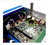
2. Insert the mSATA card into the slot at a 45-degree angle.
