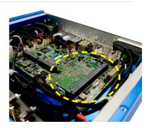
Align the notch on the memory with the key on the slot and insert the memory into the slot at a 45-degree angle.
