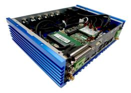
Locate the Mini PCle slot. Remove the Mini PCle card screw preinstalled on the motherboard.
