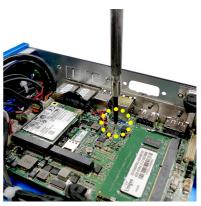
6. Insert the WiFi card into the slot at a 45-degree angle.
