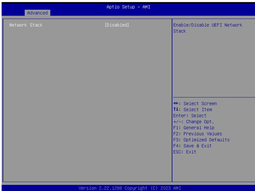
**Figure 3.33 Network Stack Configuration**
