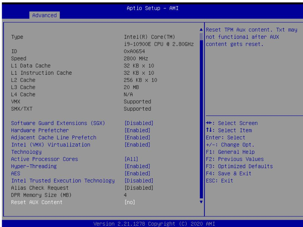
**Figure 3.6 CPU Configuration**
