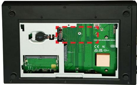
2. Unlock the SSD screw, and keep the screw for later use.
