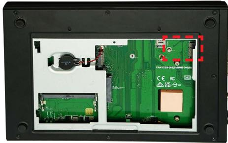
2. Unlock the M.2 card screw if needed, and keep the screw for later use.
