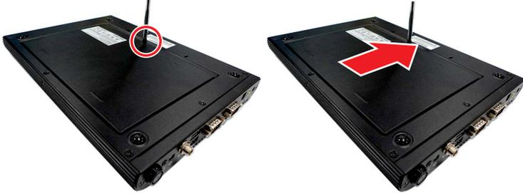
2. Remove the cover carefully, and set the cover and screw aside for later use.
