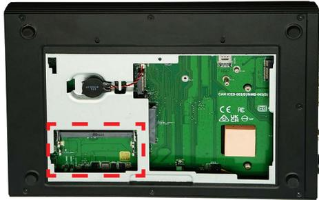
2. Align the notch on the memory module with the key on the slot and insert the memory module into the slot at a 45-degree angle.
