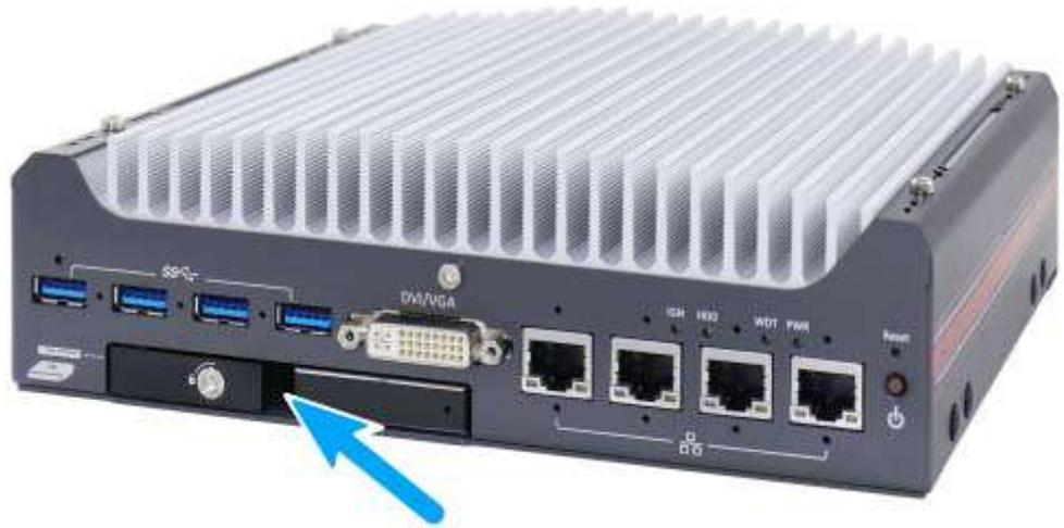
4. If you are installing a 7mm thickness HDD/ SSD, please attach the PORON materials supplied, at the corners of the non-label side, on the HDD/ SSD. With the label side facing upward, insert the SATA connector side of the 2.5" HDD/ SSD into the slot first. You may feel resistance when the SATA connectors meet, push it in firmly until the 2.5" HDD/ SSD is fully inserted into the slot.
