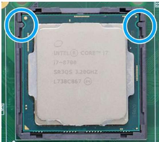
5. Locate the CPU retention bracket from the accessory box. Place the retention bracket on the CPU and hold it in place.
