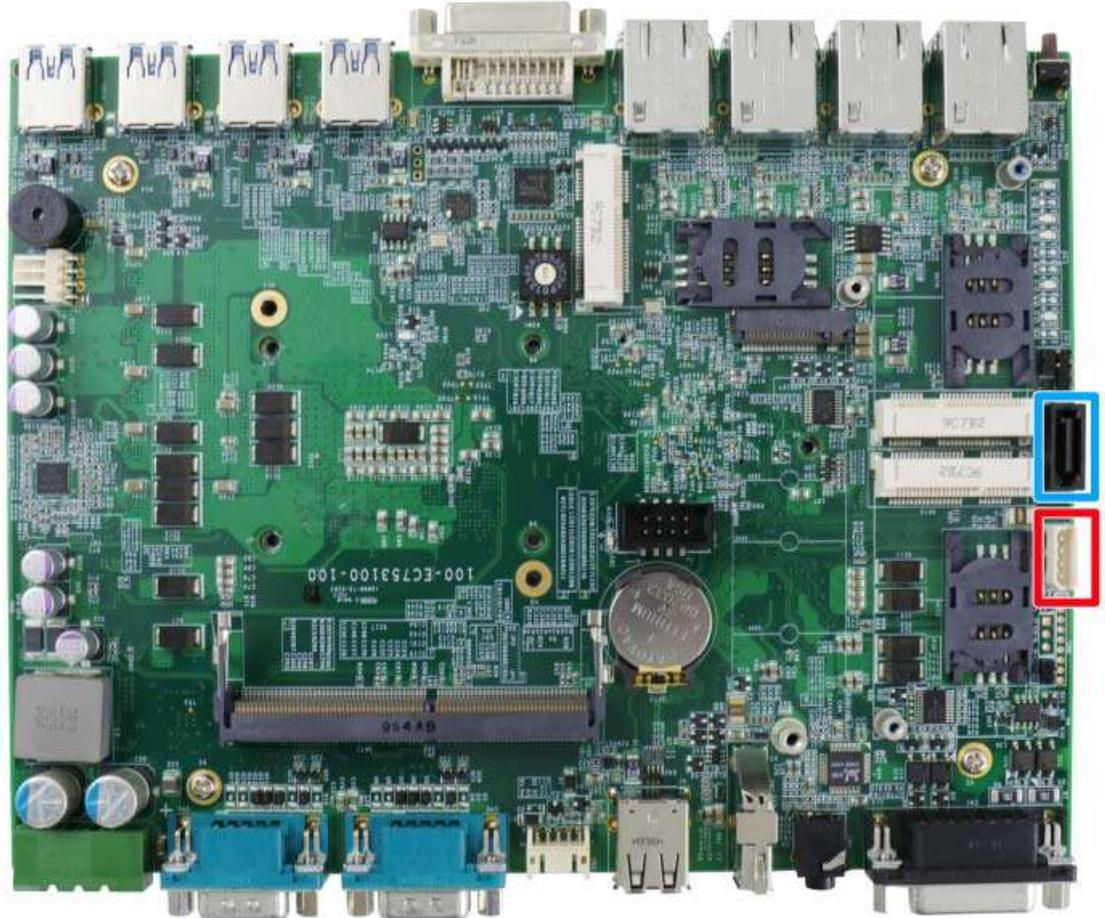
The system provides one SATA port which support Gen3, 6 Gb/s SATA signals. The SATA port is composed of a 7-pin SATA connector (indicated in blue) and a 4-pin power connector (indicated in red). This SATA and power connector should be pre-connected to the external 2.5" hot-swappable tray.
