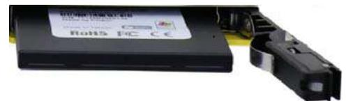
**Attach PORON on corners, on label side Insert HDD/ SSD into tray**
