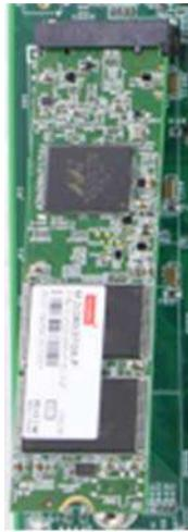
4. Gently press down and secure the module with an M3 P-head screw.
