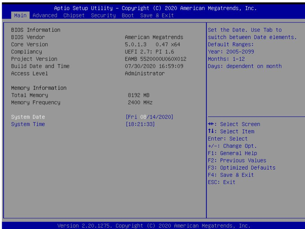
The Main setup screen has two main frames. The left frame displays all the options that can be configured. Grayed-out options cannot be configured, whereas options presented in blue can be configured. The right frame displays the key legend.
