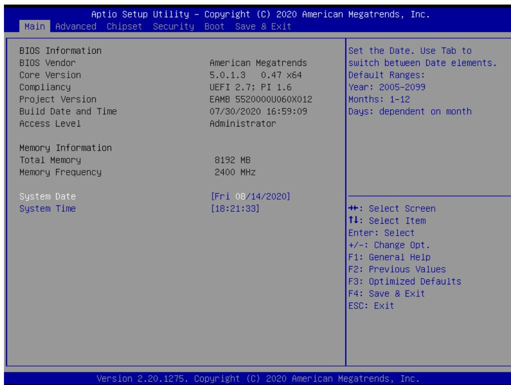
AMI's BIOS ROM has a built-in setup program that allows users to modify the basic system configuration. The setup information is stored in flash ROM to ensure it is retained when the system is powered off.
