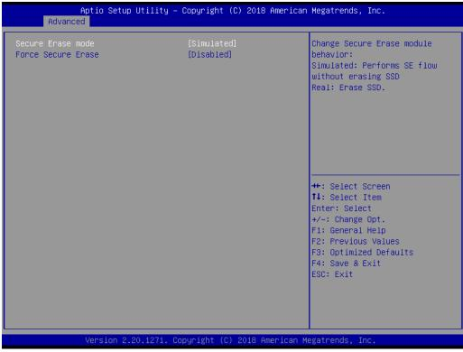
Figure 3.12 Secure Erase Configuration
