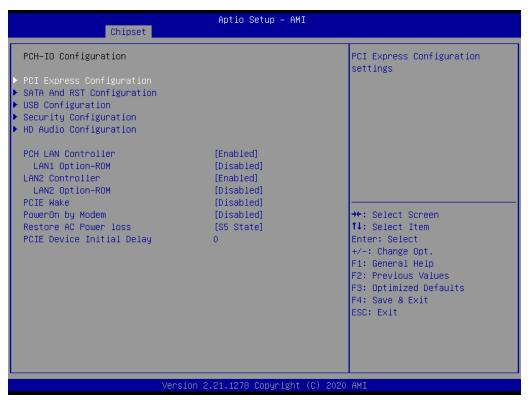
Figure 3.42 PCH-IO Configuration
