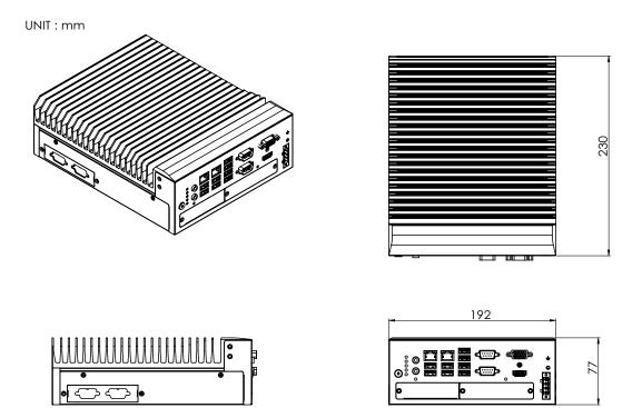
Figure 1.1 MIC-770 V2 Mechanical Dimension Drawing
