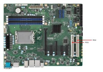
The AIMB-788 provides two 32-bit / 33 MHz PCI slots.
