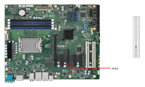
The AIMB-788 offers one PCIe x8 slot for users to install add-on cards for extension requirements. The link of PCIE3 slot is PCIe x4.
