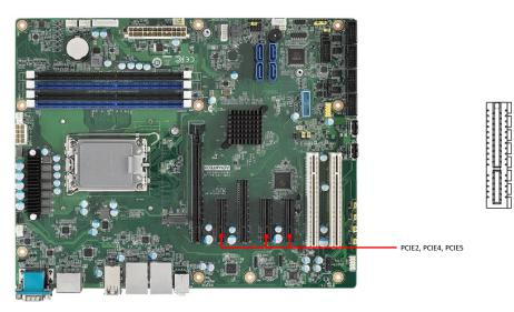
The AIMB-788 offers three PCIe x4 slots for users to install add-on cards for extension requirements.
