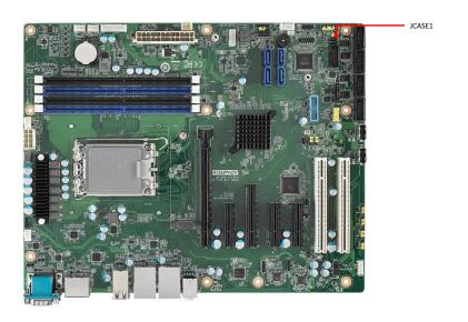
JCASE1 is for chassis with case open sensors. The buzzer on the motherboard sounds if the case is opened unexpectedly. The default function is disabled and pins 1-2 is bridged by a jumper cap.
