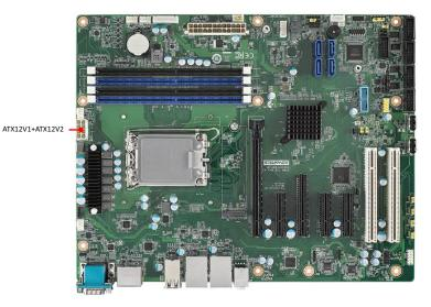
To ensure that the enough power is supplied to the CPU, one auxiliary 8-pin power connector is available on the AIMB-788. ATX12V1+ATX12V2 must be used to provide sufficient 12 V power to ensure the stable operation of the system.
