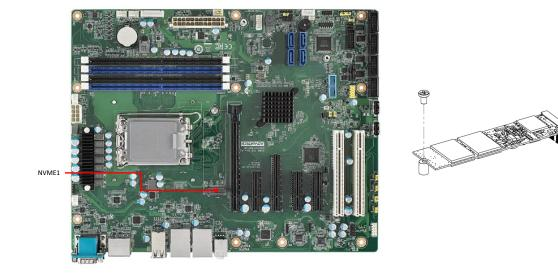
The AIMB-788 is equipped with one M.2 socket to support up to PCIe x4 M-key 2280 type storage devices. A screw to fasten the device is already installed on the nut.
