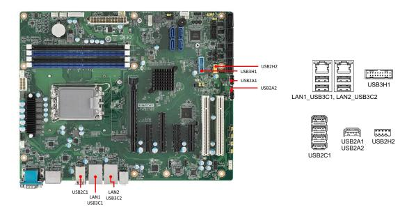
The AIMB-788 is equipped with two high-performance 1000 Mbps Ethernet LANs. They are supported by all major network operating systems. The RJ-45 jacks on the rear plate provide convenient 1000Base-T operation.
