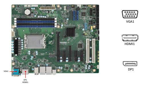
The AIMB-788 includes VGA, HDMI, and DisplayPort interface that can connect display devices. Pin assignments are detailed in Appendix B.
