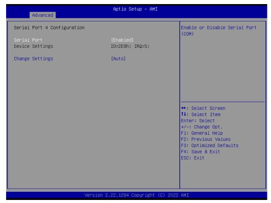
Figure 3.21 Serial Port 4 Configuration
