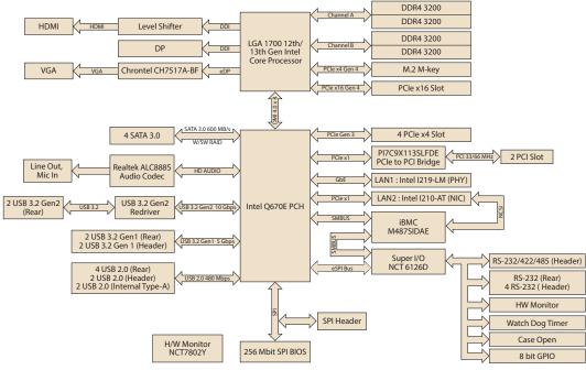
Figure 1.3 Block Diagram
