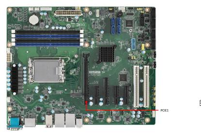
The AIMB-788 provides a PCIe x16 slot for users to install an add-on peripheral card for extension requirements. According to Intel's design specification, only graphic cards and storage cards (1x8 bifurcated PCIe 5.0, 1x4 PCIe 4.0) can be supported by the CPU PCIe port, PCIE1 slot. Other types of add-on cards installed on this slot may not have function.
