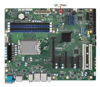
Previous LPC bus is phased out by Intel. The AIMB-788 offers SPI connector to support optional Advantech dTPM 2.0 module.
