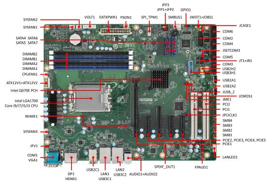
**Figure 1.1 Jumper and Connector Locations**
