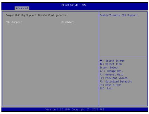
Figure 3.34 CSM Configuration
