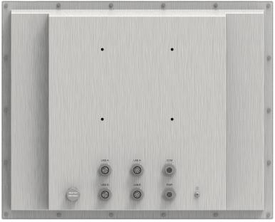
Figure 1.1 SPC-200 Rear View- I/O Port Arrangement
