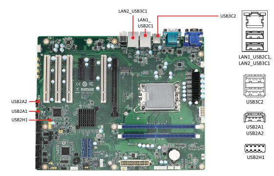
The AIMB-708 is equipped with a 1000 Mbps and a 2500 Mbps (G2 sku only) high performance Ethernet LANs. They are supported by all major network operating systems. The RJ-45 jacks on the rear plate provide convenient 1000Base-T operation. VG sku provides single GbE LAN only.
