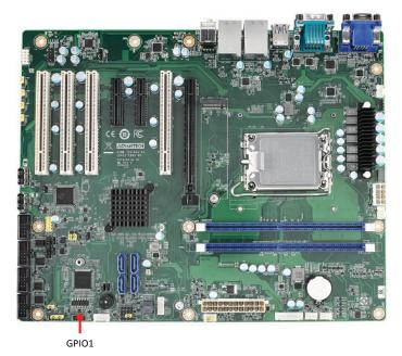
GPIO1 provides input and output connections based on your custom pin definitions.
