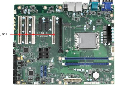
PCI4, PCI3, PCI2, PCI1
