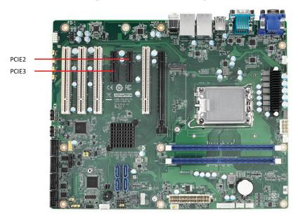
The AIMB-708 offers two PCIe x4 slots for users to install add-on cards for extension requirements. PCIE2 and PCIE3 are PCIe x1 link.
