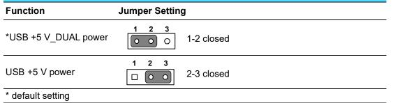
**Note!** Switching to USB +5V\_DUAL is recommended for higher stability while a KVM is used.
