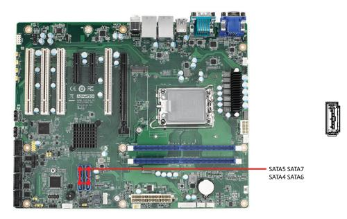
AIMB-708 features four high performance serial ATA 3.0 interfaces (up to 600 MB/s) with long, thin, easy-to-run SATA cables.
