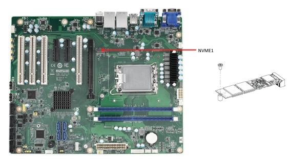
The AIMB-708 G2 sku is equipped with one M.2 socket to support up to PCIe x2 Mkey 2280 type storage devices. A screw to fasten the device is already installed on the nut.
