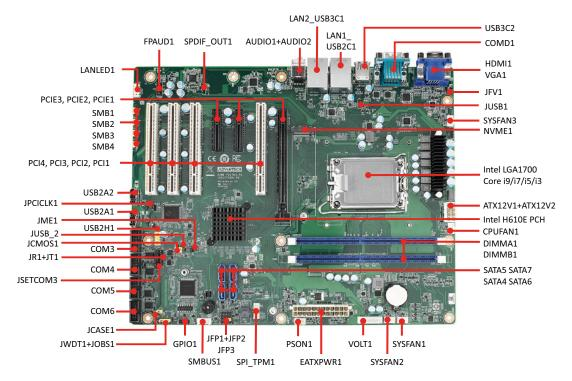
Figure 1.1 Jumper and Connector Locations
