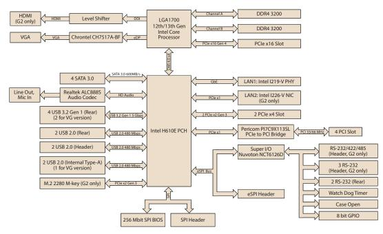
Figure 1.3 Block Diagram
