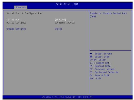
Figure 3.19 Serial Port 6 Configuration
